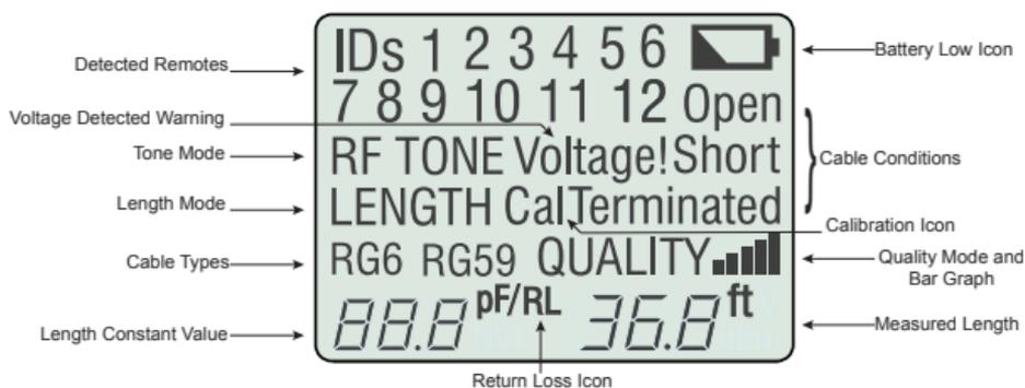
Figure 2. LCD Display Screen
