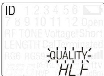
Figure 15. Poor Network Quality Error
