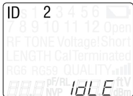
**Figure 16.** Detected ID Only Coax Remote
