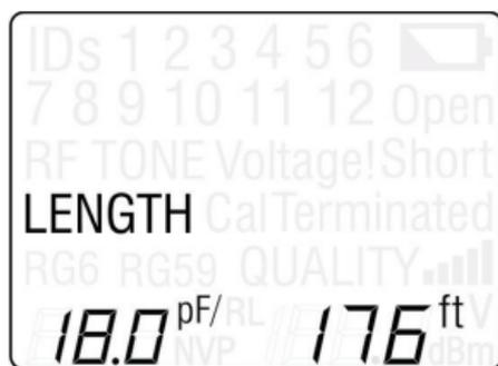
**Figure 5.** Length Measurement for Unspecified Cable
