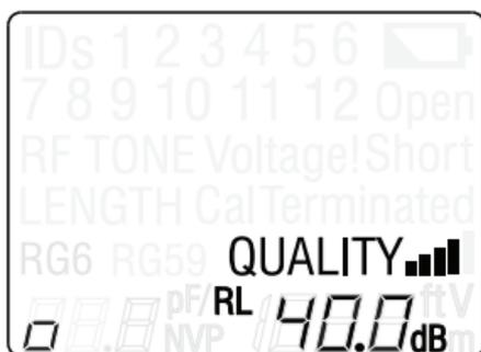
**Figure 18.** LCD Display Screen in Quality Mode
