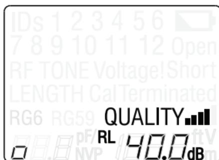
**Figure 6.** Return Loss Measurement in Quality Mode
