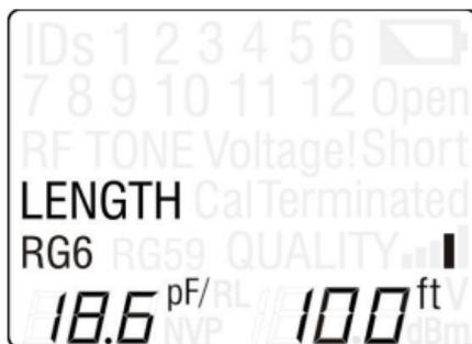
**Figure 12.** Measured Cable Length
