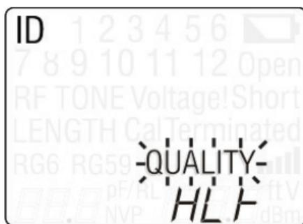
**Figure 4.** ID Mode with Poor Network Quality
