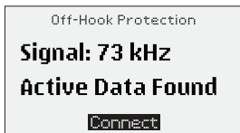
Figure 4.4 Data Present Warning
