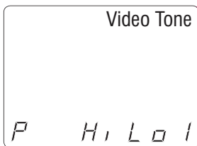
Figure 12. Video Cable Test with Pin Selected
